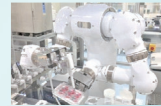
Human-type robot for general-purpose experiments "Maholo"
